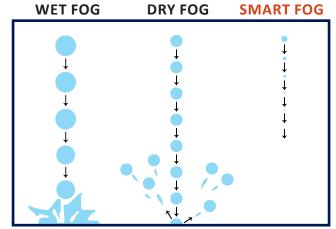
Wet Fog droplets burst and wet the surfaces, like rain.
